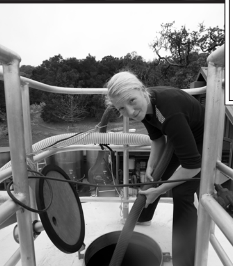
Pump-over under macerationen
